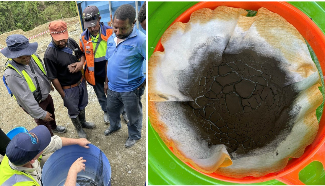
Figure 2: Gold precipitate being recovered by decanting and filtration.
