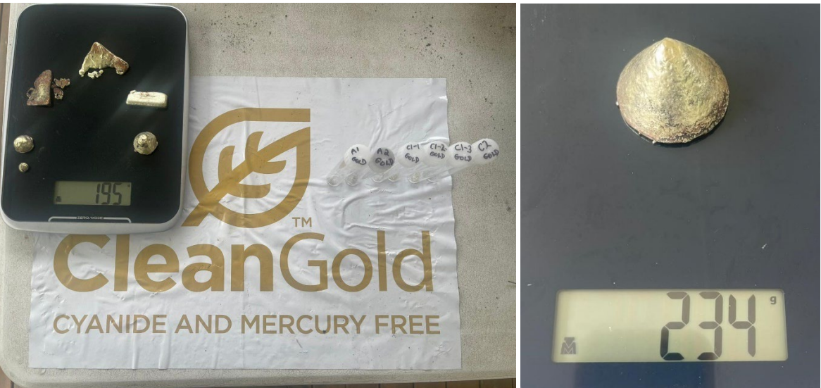
Figure 3: Gold dore products – some individual test products on the left and final combined product on the right.
